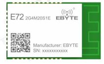
The module leads all the IO ports of the single-chip microcomputer. The chip comes with a powerful 48 MHz Arm & Cortex & -M4F processor, an internal
