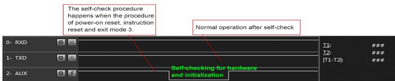
Timing Sequence Diagram of AUX when self-check
