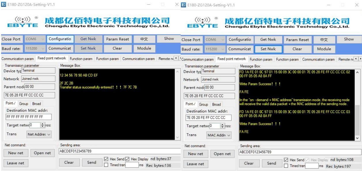
(2) After the target MAC address is configured, the transmission mode needs to be configured. Change the "network address (short address)" to "MAC address", and then write the parameters again. At this time, the target address is configured to unicast in the form of MAC address.
