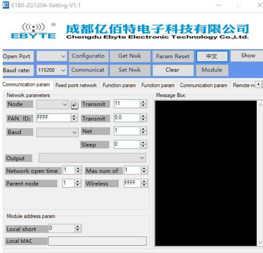
(2) After the serial port is opened, first click “Enter Configuration Mode”, the message box prompts “Enter the configuration status successfully, read parameters successfully”. The main network parameters include: the node type defaults to the end-device, the channel 11 (default), the PAN ID defaults randomly, and the transmit power is 20. (default)
