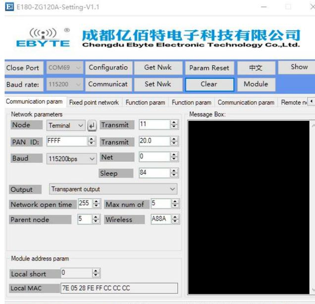
(3) Modify node type as coordinator, and click the Enter button, the message box prompts "Configure device type success". The general ZigBee 3.0 network is established by the coordinator node, so the factory default end-device node type needs to be changed to the coordinator before establishing the network.
