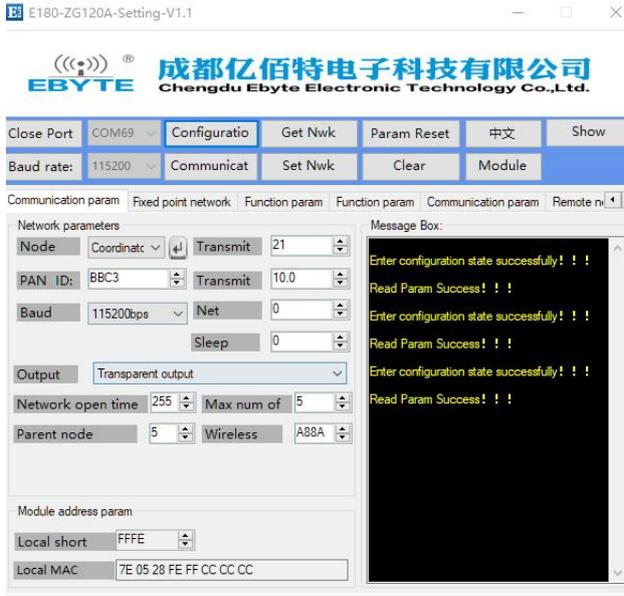
(7) Select the fixed-point networking interface, display the network status as "joined network". The coordinator network is successfully created.
