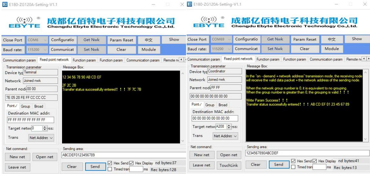
7.3.1.2 Unicast in long address form between end-device and coordinator
