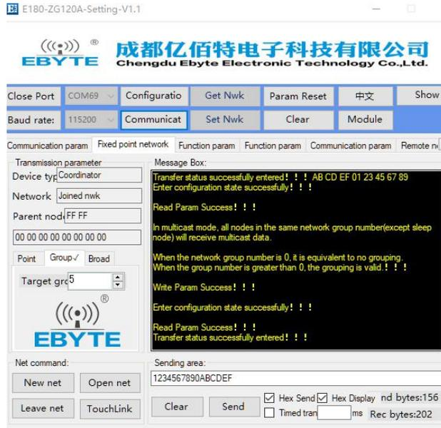
(3) Enter the transmission mode, the message box will prompt "enter the transmission mode successfully", and then carry out multicast data communication.
