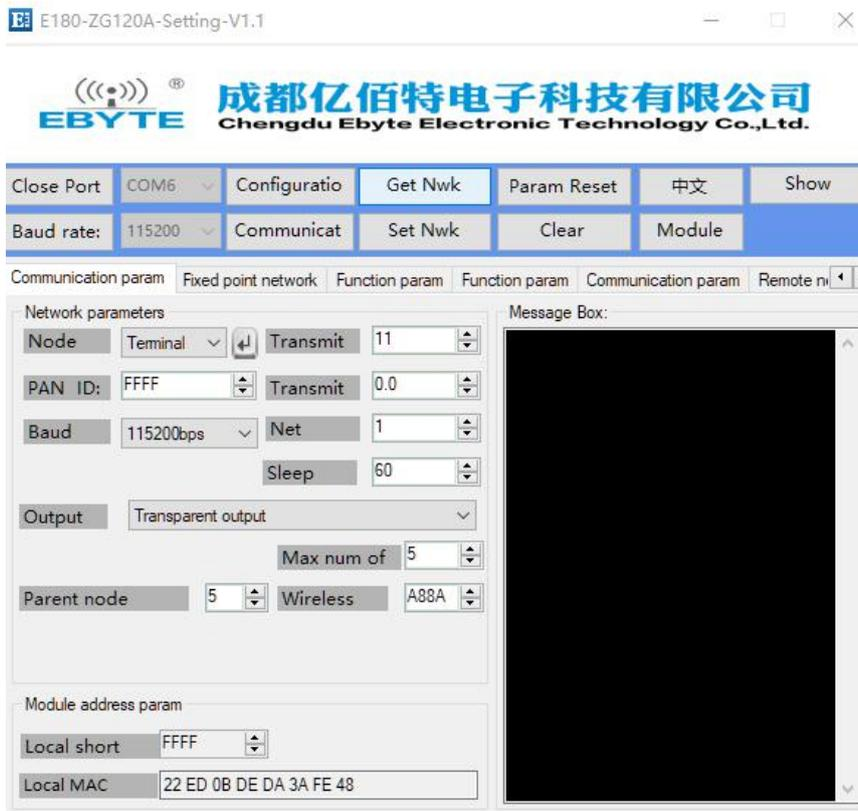
(3) Modify the node type as sleep-end-device, click the Enter button, the message box prompts "Configure device type is successful", modify the network parameters, its PAN ID and transmit channel parameters must be the same as the network to be joined, click "Write network parameters", The message box prompts "Write parameters successfully."
