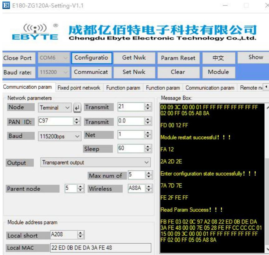
(5) Select the fixed-point networking interface and display the network status as “joined network”. The sleep-end-device node has joined the network created by the former coordinator.
