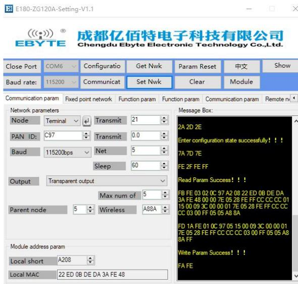
(2) For example, if the coordinator is the sender, click "enter configuration mode" to enter the fixed-point networking, select the multicast mode, and the message box will prompt "under multicast mode, all nodes with the same group number in the network will receive multicast data", modify the target group number to "5", and then write the parameter, and the message box will prompt "write the parameter successfully".
