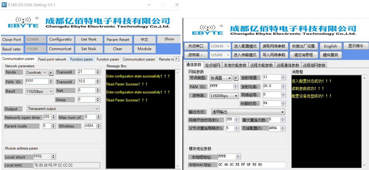
(4) After the node type is successfully written, modify the ZigBee network required for establishing some network parameters (you can also use the default value without modifying the parameters). Modify the channel, network PANID and transmit power. After modifying the parameters, click "Write Network Parameters". ", the message box will prompt "Write parameters successfully"
