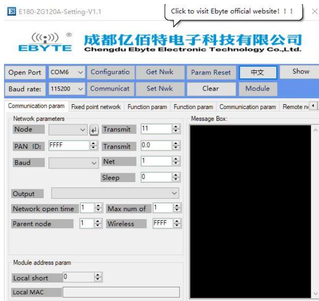
(2) After the serial port is opened, first click “Enter Configuration Mode”, the message box prompts “Enter the configuration status successfully, read parameter successfully”. The main network parameters include: the node type defaults to the end-device, channel 11(default), PAN ID random (default), transmit power is 10 (default).
