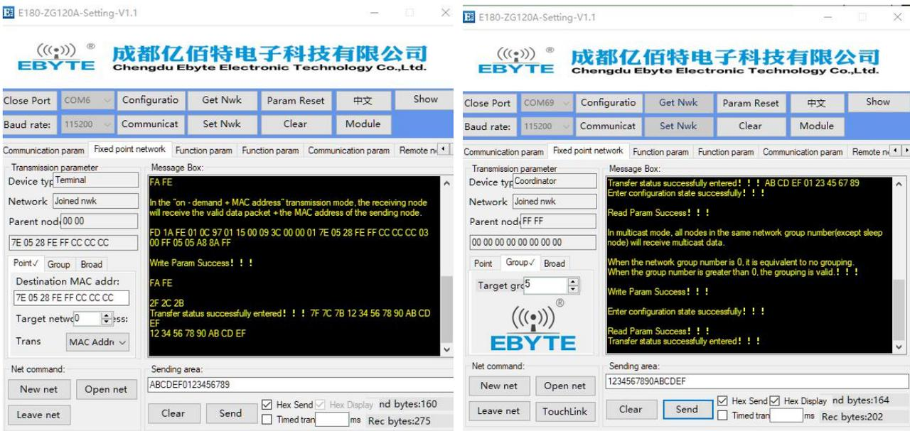
(4) The end-device receiver enters the configuration mode, changes the network group number to "4", and writes the parameter. At this time, because the network group number is not "5", the coordinator multicast data cannot be received.
