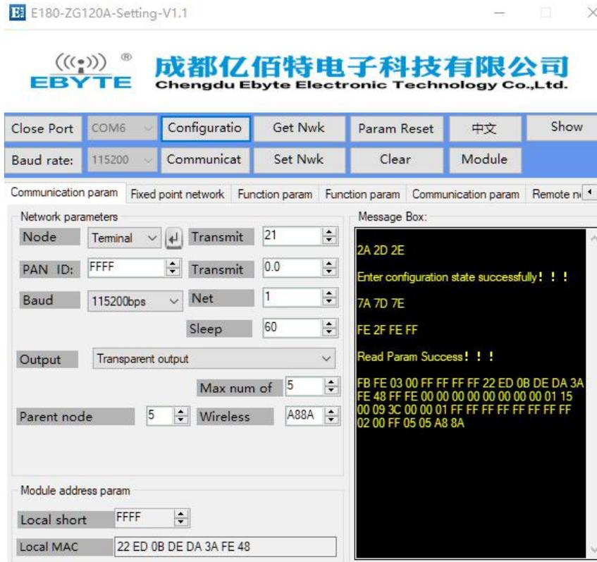
(4) Click "Module Restart", the message box prompts "Module restart is successful", click "Enter configuration mode", the message box prompts "Enter configuration status is successful, read parameters successfully", confirm whether the read PAN ID and transmit channel parameters are Modified value before.
