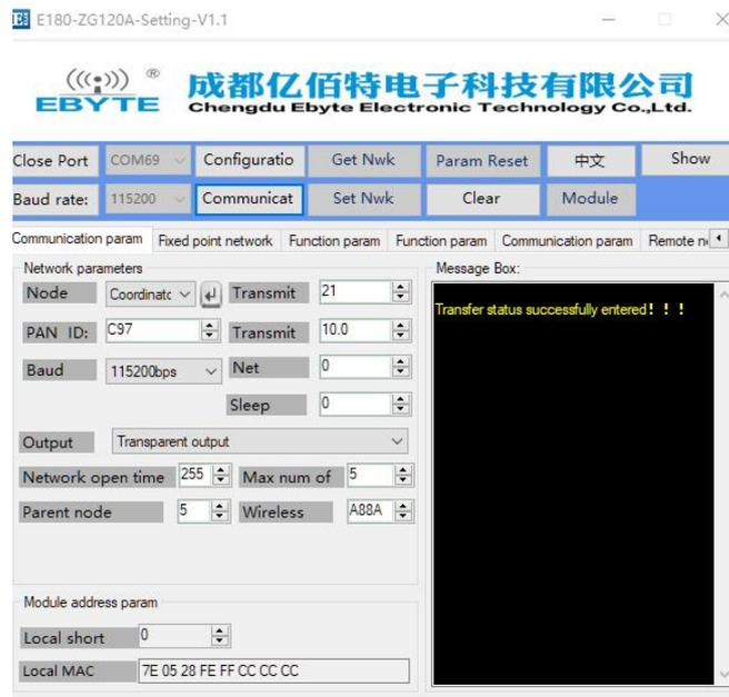
(6) After the module restarts, the transfer mode is entered by default. At this time, click “Enter Configuration Mode” again, the message box prompts “Enter the configuration status successfully, read parameters successfully”. It can be seen that the parameters read out are the previously modified parameters, indicating that the network parameters are modified successfully.
