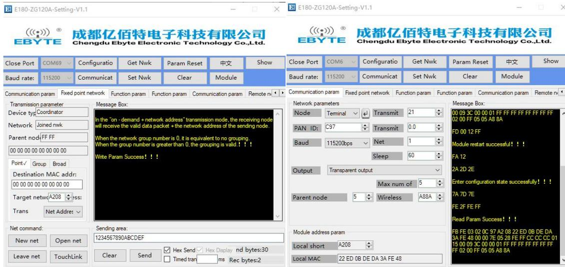
(2) After the target address between nodes is configured, click "enter transmission mode", and the message box will prompt "enter transmission mode successfully". Before communication, confirm whether the module is in transmission mode, and only in the transmission mode can the communication be realized. Input the data to be sent in the sending area, click send, and the received data can be seen in the end-device node message box.
