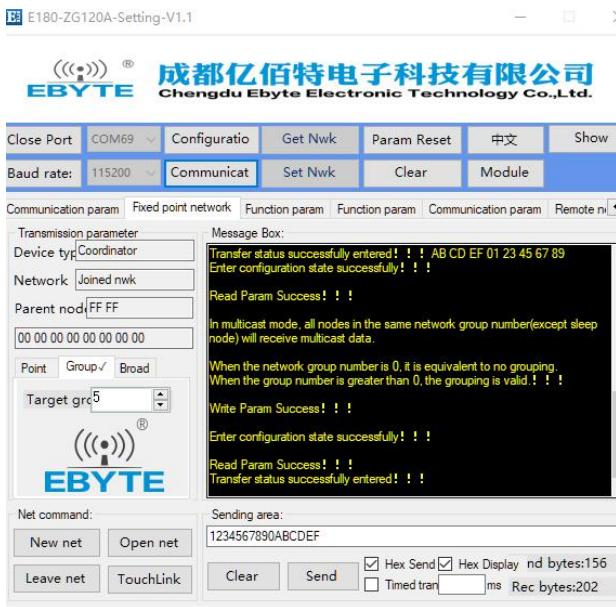
(3) Enter the transmission mode, the message box will prompt "enter the transmission mode successfully", and then carry out multicast data communication.
