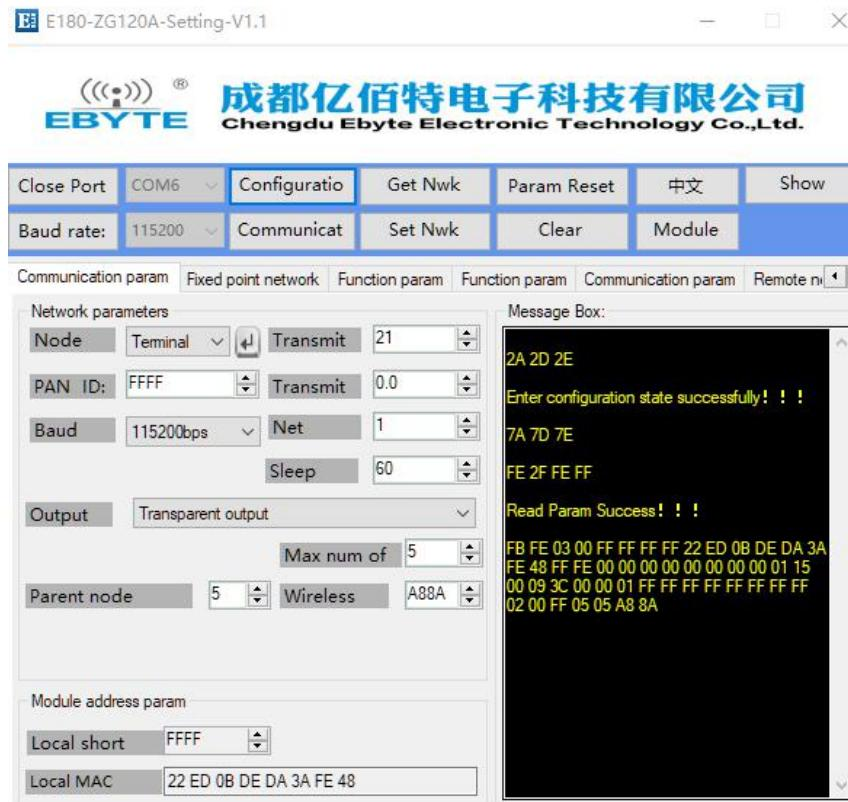
(4) Click "Module Restart", the message box prompts "Module restart is successful", click "Enter configuration mode", the message box prompts "Enter configuration status is successful, read parameters successfully", confirm whether the read PAN ID and transmit channel parameters are the modified value before.(PAN ID of the established network coordinator).
