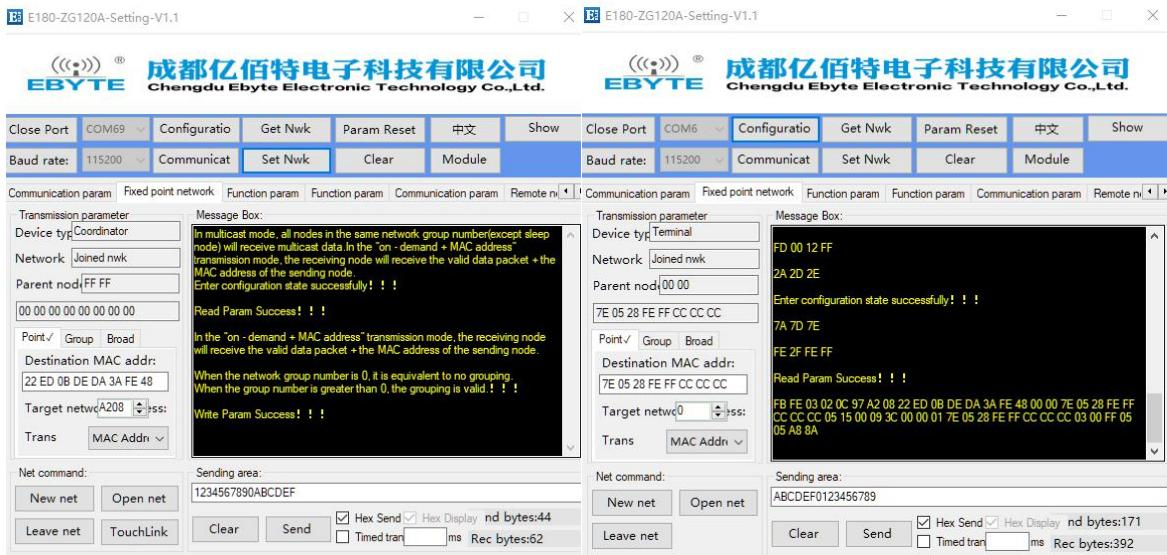
(3) After completing the above parameter configuration, click to enter the transmission mode, communicate in the transmission mode.
