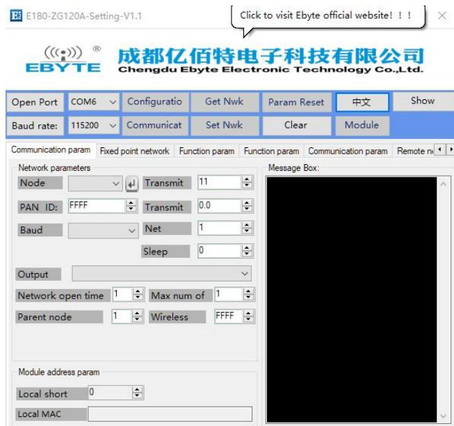
(2) After the serial port is opened, first click “Enter Configuration Mode”, the message box prompts “Enter the configuration status successfully, read parameter successfully”. The main network parameters include: the node type
