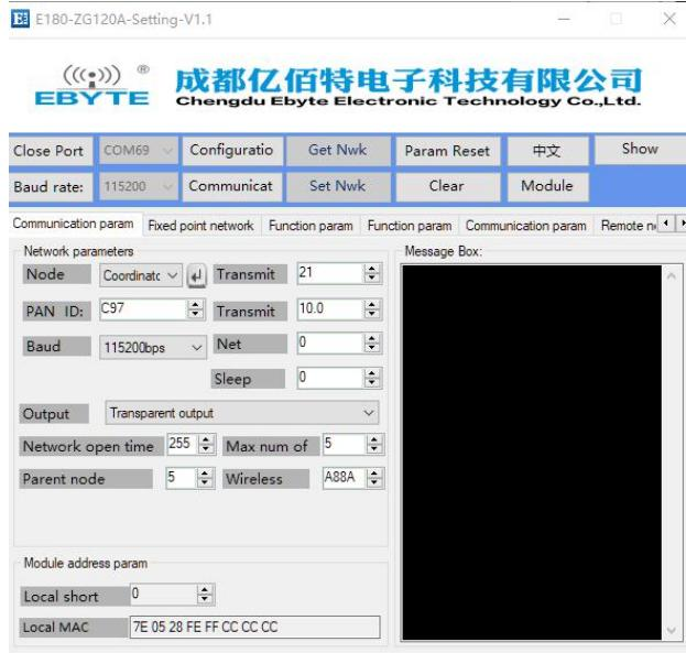
(5) After the node type is modified, the module needs to be restarted to take effect. Click “Module Restart”, and the message box prompts “Module restart successful”.
