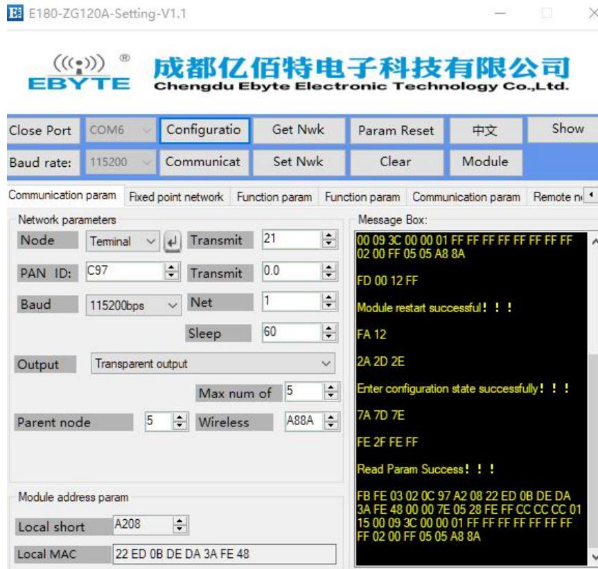
(5) Select the fixed-point networking interface and display the network status as “joined network”, indicates sleep-end-device node has joined the network created by the former coordinator.
