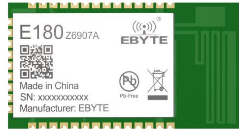
TLSR8269 is a wireless microcontroller for smart home, IoT transformation and industrial automation. Its network characteristics belong to ZIGBEE 3.0 standard and provide a complete application integration solution based on IEEE802.15.4 standard ISM band.
