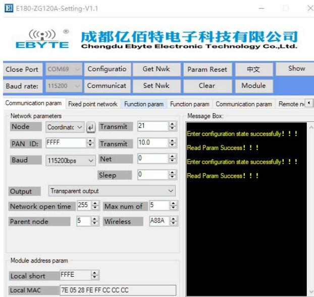
(4) After the node type is successfully written, modify the ZigBee network required for establishing some network parameters (you can also use the default value without modifying the parameters). Modify the channel, network PANID and transmit power. After modifying the parameters, click “Write Network Parameters”. , the message box will prompt "Write parameters successfully".
