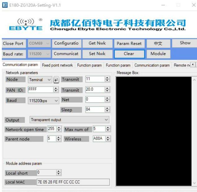
(3) Modify node type to coordinator, and click the Enter button, the message box prompts "Configure device type successfully". The general ZigBee 3.0 network is established by the coordinator node, so the factory default end-device node type needs to be changed to the coordinator before establishing the network.
