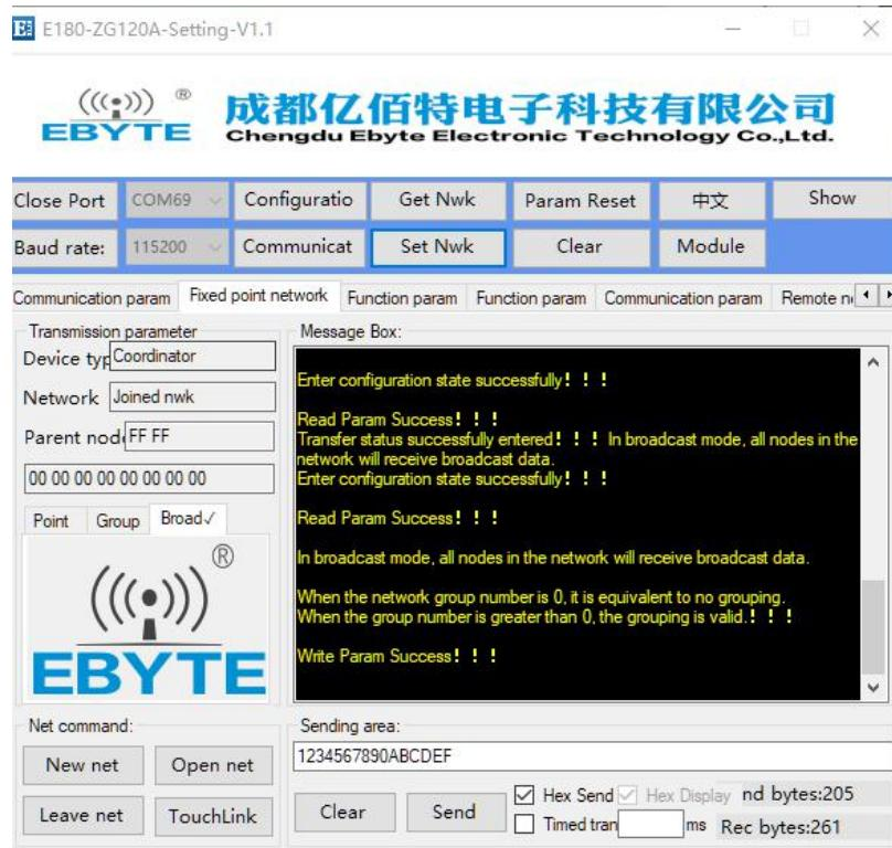
(2) Enter the transmission mode, the message box will prompt "enter the transmission mode successfully", and then broadcast data communication, at this time, all nodes in the network will receive data, including the sending node.
