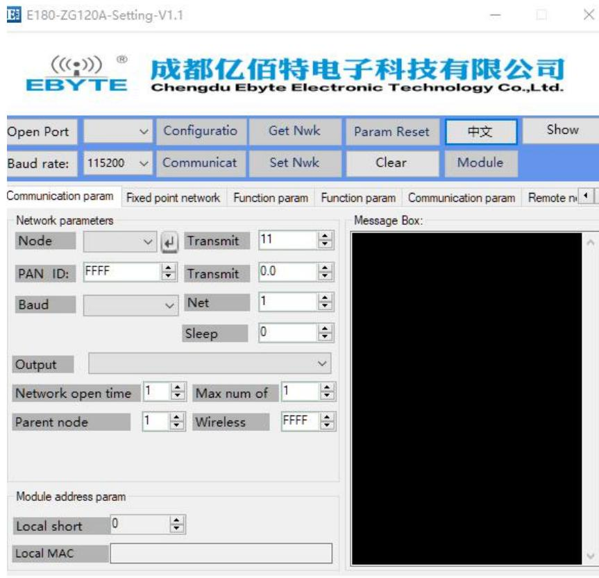
(2) After the serial port is opened, first click “Enter Configuration Mode”, the message box prompts “Enter the configuration status successfully, read parameters successfully”. The main network parameters include: the node type defaults to the end-device, the channel 11 (default), the PAN ID defaults randomly, and the transmit power is default 0 (7dbm).
