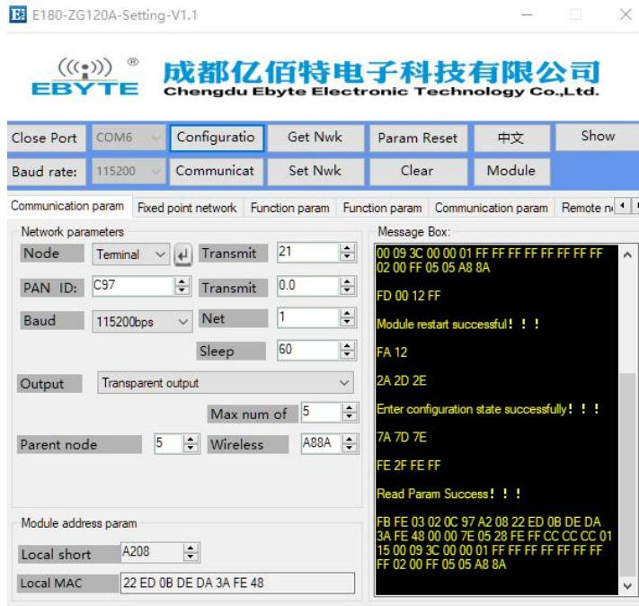
Similarly, the end-device node also join the ZigBee network according to the above method. If the node type does not need to be added to another ZigBee network, the Enter button next to the node type configuration also needs to be clicked. Write the parameters after modifying the network parameters, and finally restart to join the new ZigBee network.
