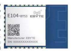
This module is a pure hardware SoC module without firmware program. The functions of Bluetooth-based broadcasting, scanning, connection, and transparent transmission can only be realized after the user's secondary development.
