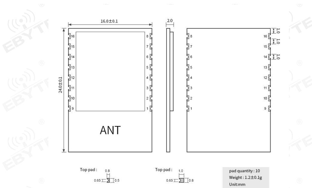
Figure 3-1 Mechanical size and pin definition
