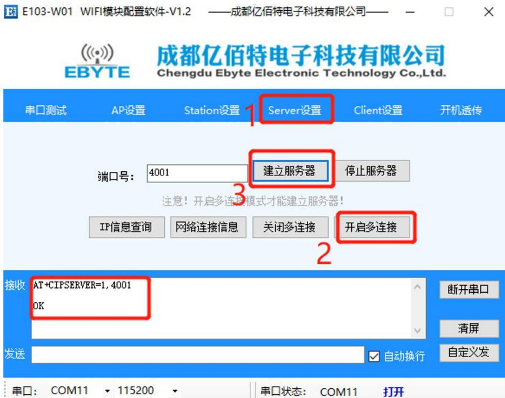
⑥ We build a client on the PC and connect to the client of the module, and then we can send data. Here, if the server needs to send data to the client, we can send it through the AT+CIPSEND command. Here, users can download the AT instruction manual of E103-W05 in the data download.
