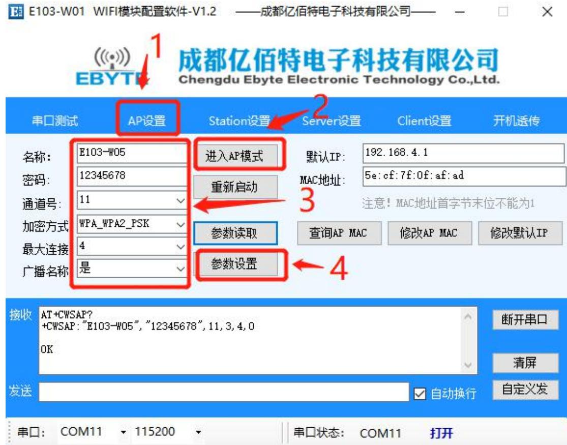
③ After the setting is successful, we can search through the WIFI in the lower right corner of the computer to find our module and connect it.
