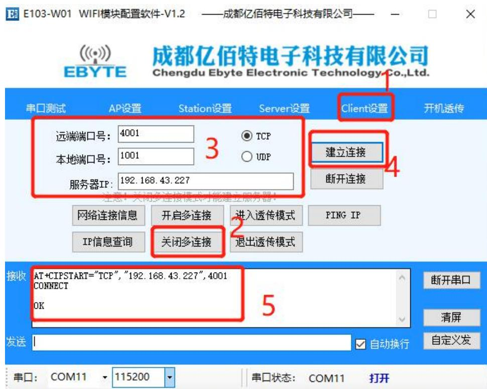
⑤After successfully connecting to the server, we can perform data communication between the server and the client, but here, in order to achieve simple data transmission, we need to make some settings to enter the transparent transmission mode, so that we can avoid sending data every time. The awkward operation of specifying the width. After the client connects to the server, perform the following operations to enter the transparent transmission.
