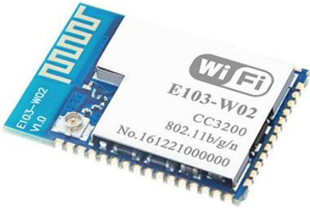
E103-W02 is a ultra low power UART to Wi-Fi module with small size SMT packing and embeded PCB antenna, operating at 2.4 ~ 2.484GHz. The module can transmit and receive data through UART, which makes it easier for wireless applications.
