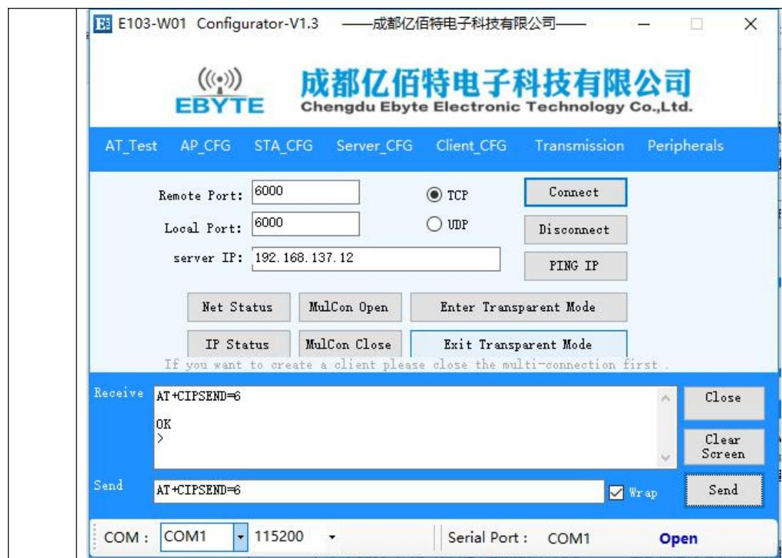
After ">" symbol shows, transmit data "123456" , user can see the TCP server receive data "123456".
