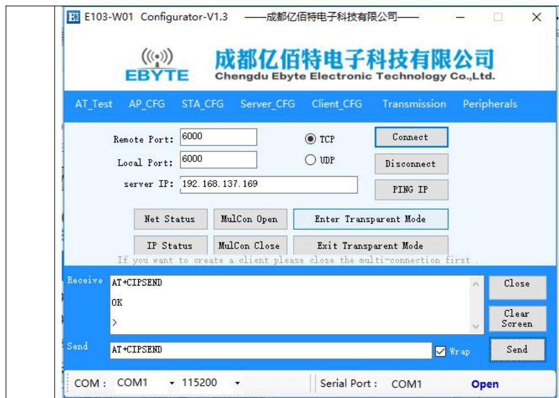
Notes: module no longer receive AT command, transmit the data from UART to server directly.
