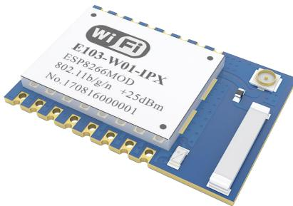
E103-W01-IPX is 100mW (20dBm) UART-WiFi module with competitive price. It is small-size with both IPX and embedded PCB antenna, operating at 2.4~2.4835GHz, and very easy for user to operate.
