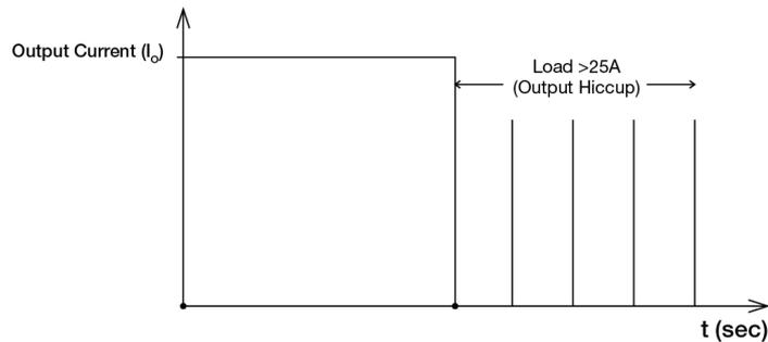
It is not recommended to prolong the duration of  $I_o$  when it is <25A but >14.6A, since it may cause damage to the PSU.
