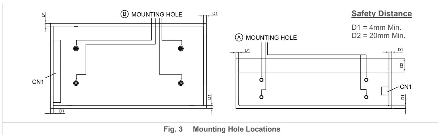
Ensure the mounted device is kept at  $\geq 4$  mm (0.16 inch) safety distance at all sides from other components and equipments. In addition, to ensure sufficient convection cooling, always maintain a distance of  $\geq 20$  mm (0.79 inch) from fan ventilated surfaces while the device is in operation. Please insert an insulation sheet between the system and product, if the safety distance is  $< 4$  mm (0.16 inch).
