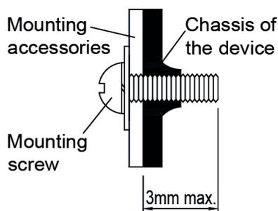
Fig. 4 Mounting Screw
