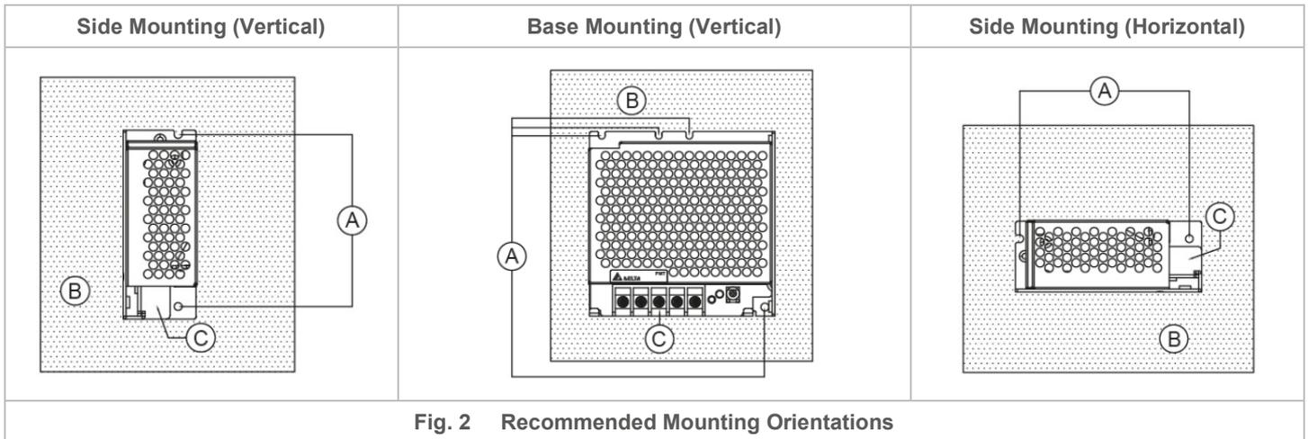
Fig. 2 Recommended Mounting Orientations
