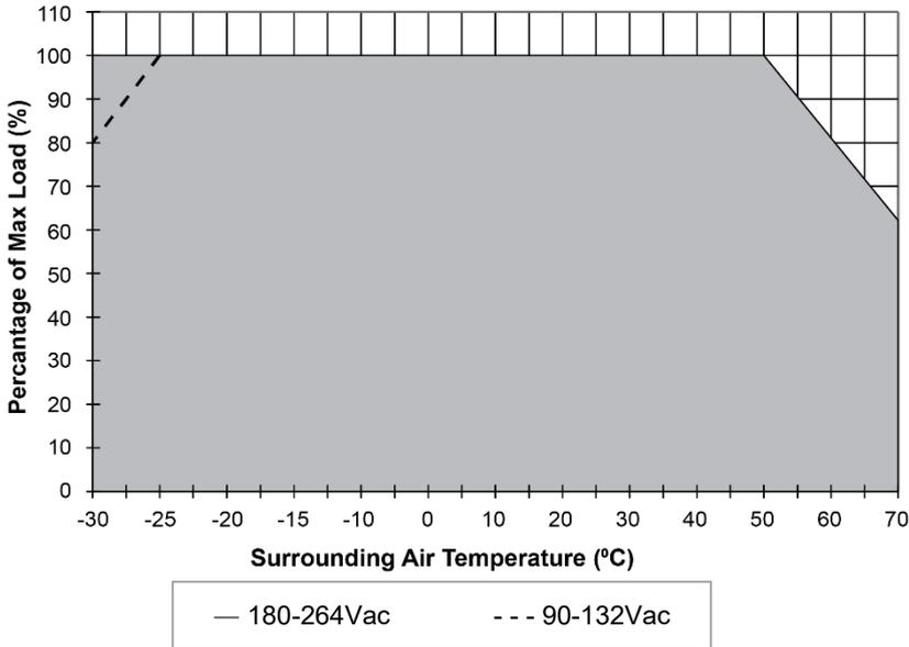
**Fig. 1 De-rating for Horizontal Mounting Orientation**
