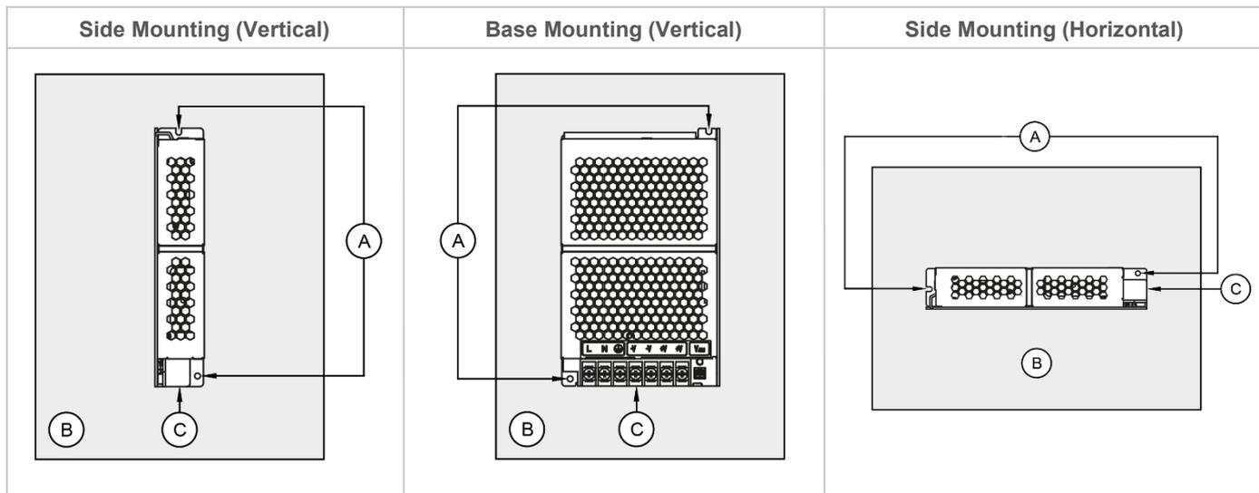
Fig. 2 Mounting Orientation
