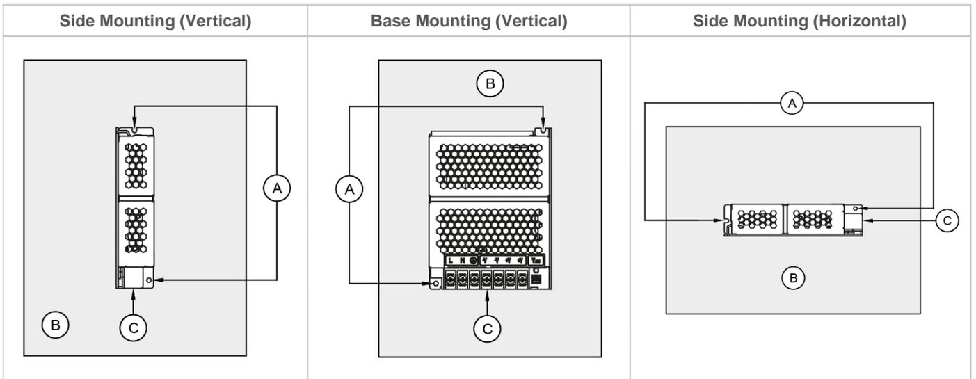
Fig. 2 Mounting Orientation
