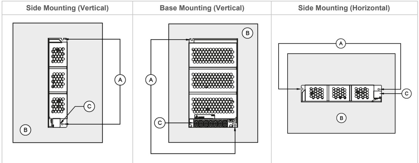
Fig. 2 Mounting Orientation
