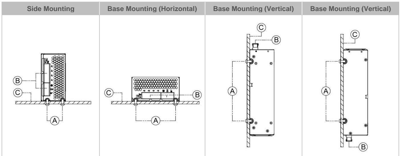
Fig. 2 Mounting Orientation
