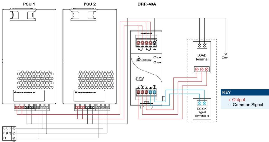
Fig. 3 Redundancy / Parallel Operation Connection Diagram
