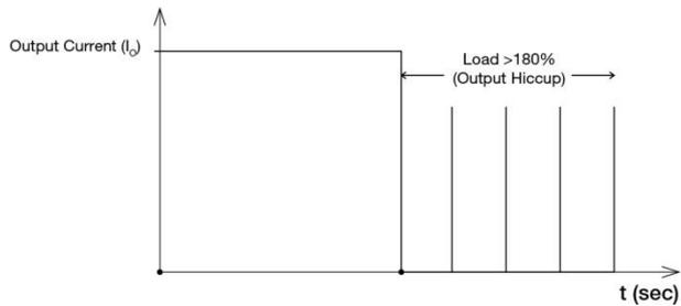
It is not recommended to prolong the duration of  $I_o$  when it is <180% but >100%, since it may cause damage to the PSU.
