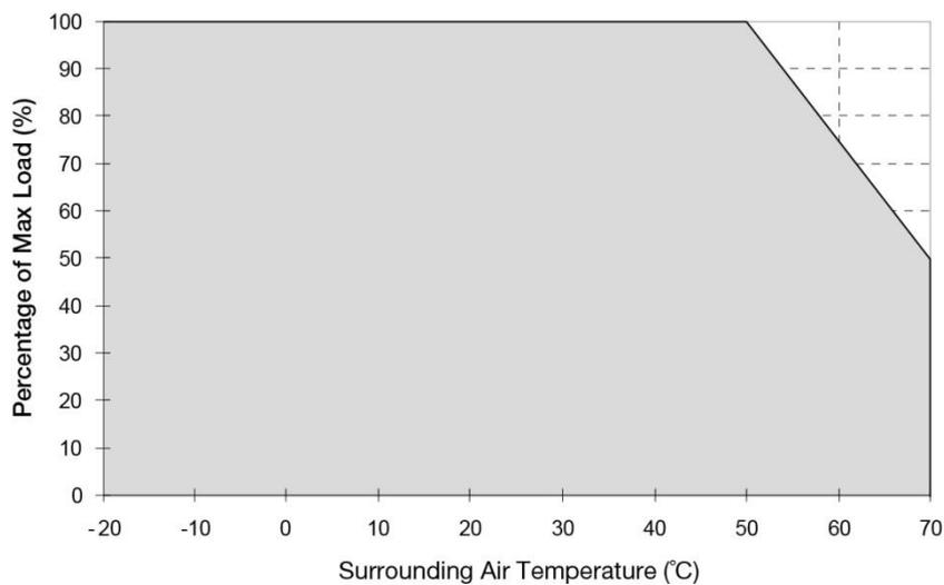
**Fig. 1 De-rating for Vertical and Horizontal Mounting Orientation**
