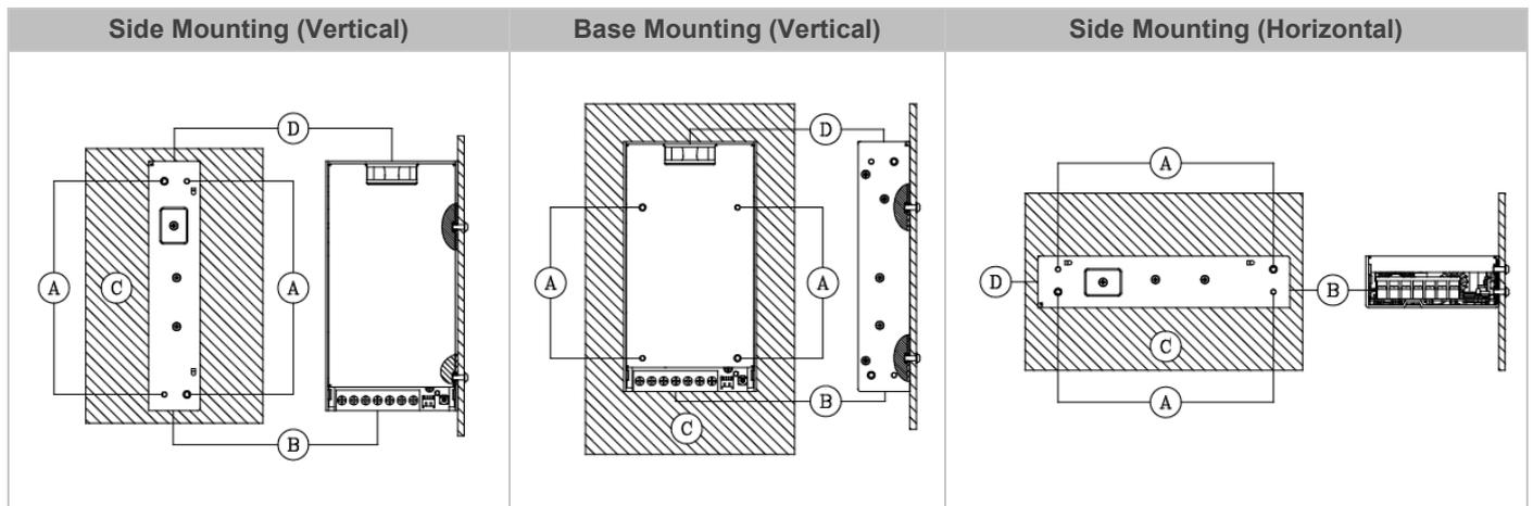
Fig. 2 Mounting Orientation
