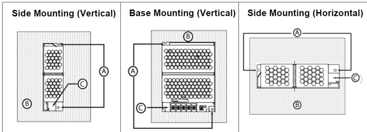
Fig. 2 Mounting Orientation
