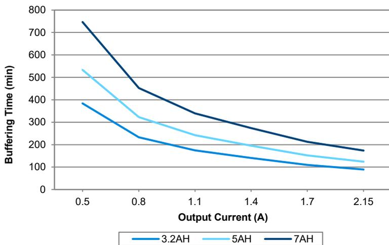
Fig. 2 Buffering Time VS Output Current (PJU-27V60W□□□)
