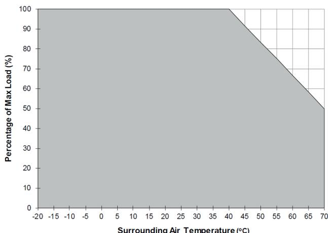
**Fig. 3.3 De-rating for Horizontal Base Mounting**
