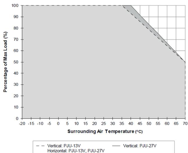
**Fig. 3.1 De-rating for Vertical Base Mounting**
