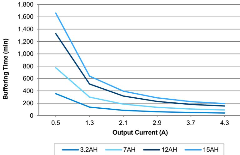
Fig. 1 Buffering Time VS Output Current (PJU-13V60W□□□)
