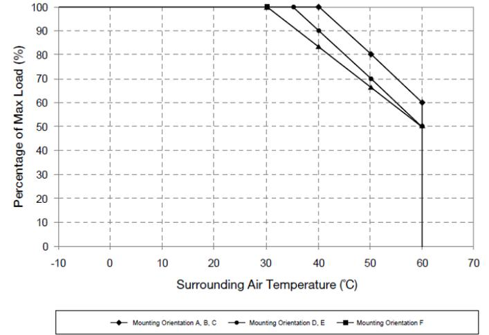
Fig. 1.2 De-rating for Mounting Orientation A, B, C
