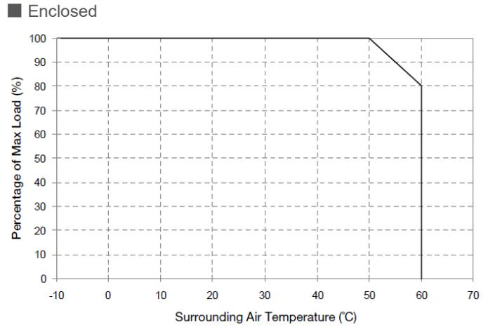
Fig.1.4 De-rating for Mounting Orientation A to F
