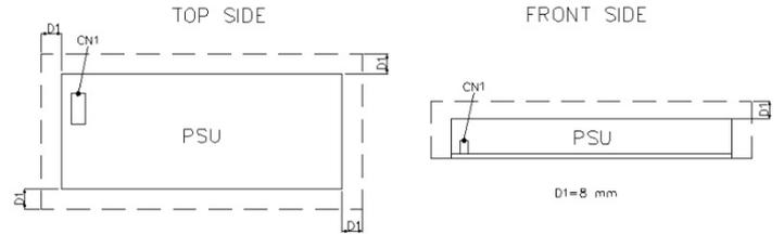
For safety reasons, please ensure the mounted device is kept at  $\geq 8\text{mm}$  (0.315 inch) safety distance at all sides from other components and equipments. **Please insert an insulation sheet between the system and product, if the safety distance is less than 8mm (0.315 inch).**
