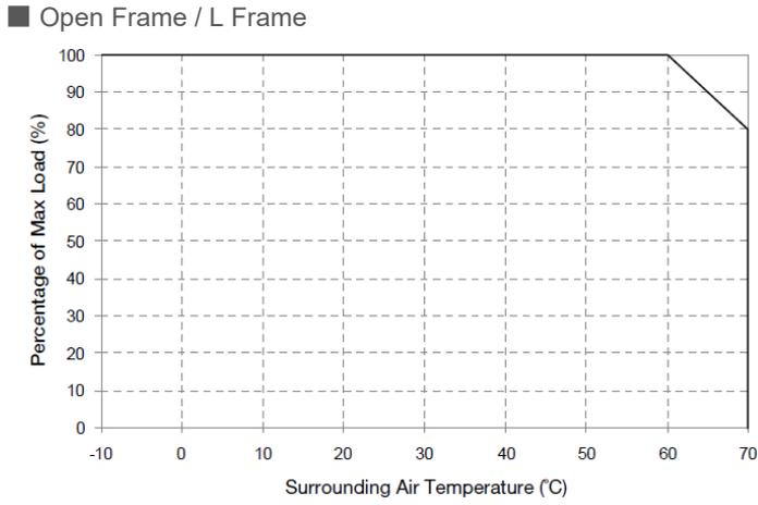
Fig.1.3 De-rating for Mounting Orientation A to F
