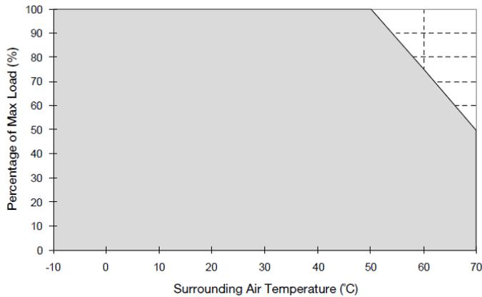
Fig.1.1 De-rating for Mounting Orientation A to F
