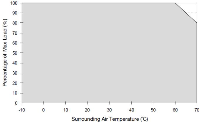
Fig.1.3 De-rating for Mounting Orientation A to F
