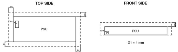
For safety reasons, please ensure the mounted device is kept at  $\geq 4\text{mm}$  (0.16 inch) safety distance at all sides from other components and equipments. **Please insert an insulation sheet between the system and product, if the safety distance is less than 4mm (0.16 inch).**
