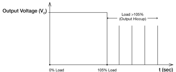
It is not recommended to prolong the duration of  $I_o$  when it is  $<105\%$  but  $>100\%$ , since it may cause damage to the PSU.
