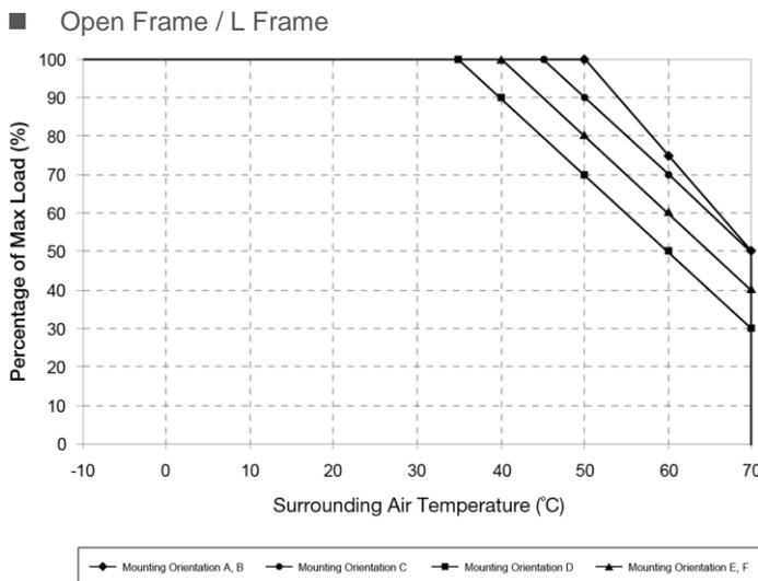
Fig.1.1 De-rating for Mounting Orientation A, B
