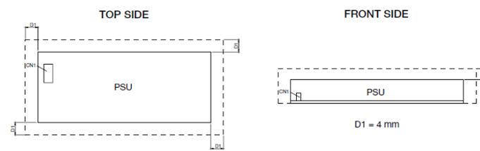
For safety reasons, please ensure the mounted device is kept at  $\geq 4$ mm safety distance at all sides from other components and equipments. **Please insert an insulation sheet between the system and product, if the safety distance is less than 4mm.**
