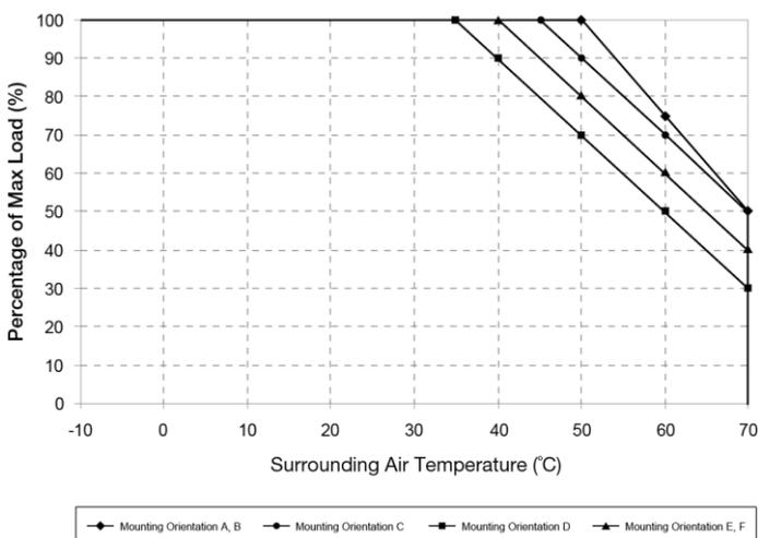
Fig.1.1 De-rating for Mounting Orientation A, B
