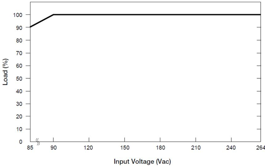
■ No output power de-rating for the input voltage range from 90Vac to 264Vac
