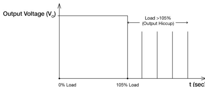
Additionally, if the  $I_o$  is <105% but >100% for a prolong period of time (depending on the load), the Over Temperature Protection (OTP) will be activated due to high temperature on critical components. The power supply will then go into latch mode until the fault is removed and the mains is reapplied.
