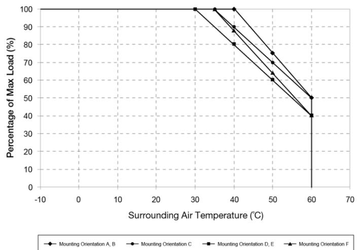
Fig.1.2 De-rating for Mounting Orientation A, B
