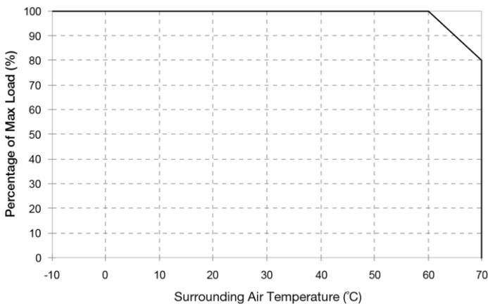
Fig.1.3 De-rating for Mounting Orientation A to F
