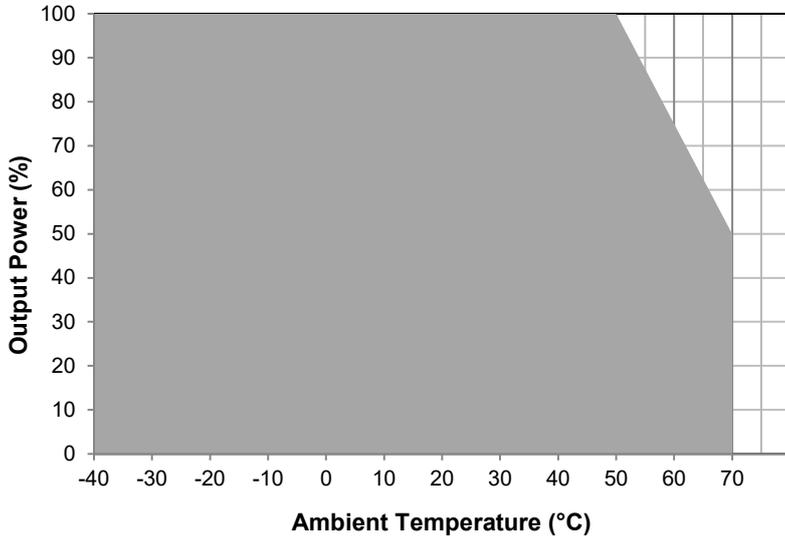
**Fig. 1 De-rating for All Mounting Orientation**
