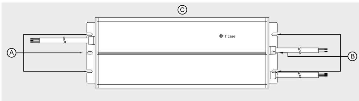
Fig. 3 Mounting Hole Locations
