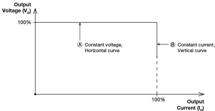
A typical LED power supply is able to either work in "constant voltage mode (CV) or constant current mode (CC)" to drive the LEDs. Delta's LNE drivers integrate CV+CC characteristics; so operation in CV mode (with external LED driver), in region (A) or CC mode (direct drive, at area (B)).
