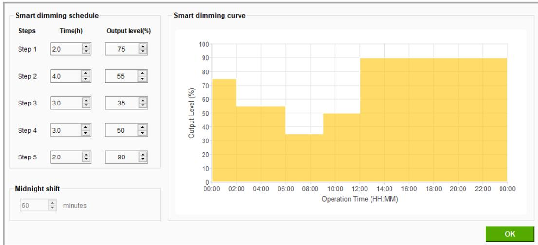
**Midnight Centric Timer:** This mode is a memory-based that automatically measures over the past two days the power-on time of the lighting installation at which is the naturally corresponded to night time. The Midnight Centric Timer software calculates the length of power on time and centralized from the given virtual midnight point and change the output level accordingly.
