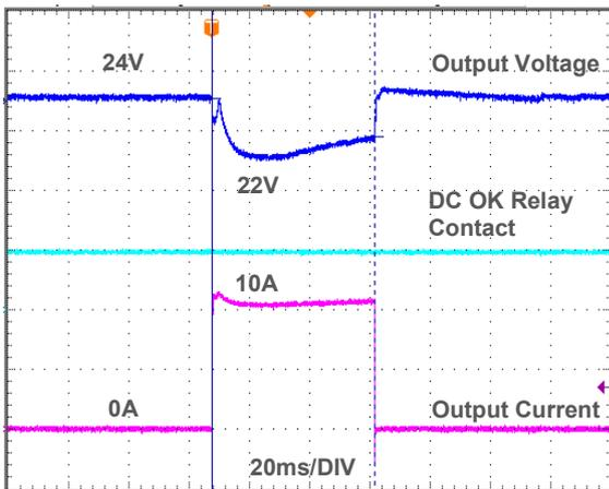
Fig. 8.1 APB 200% of nominal output current for 50ms
