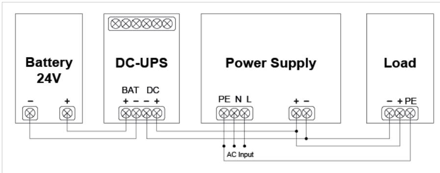
Fig. 4.2 Can be combined with redundancy module (DRR-40A)
