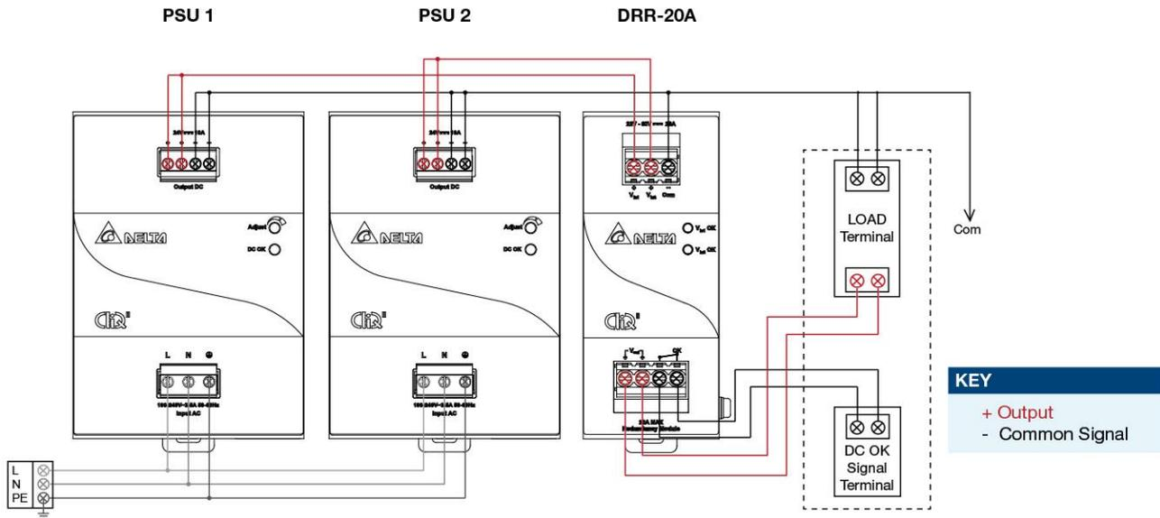
Fig. 4 Redundancy / Parallel Operation Connection Diagram
