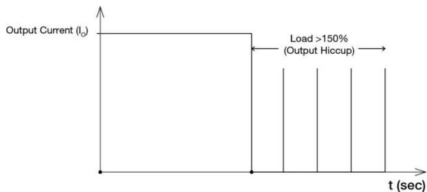
It is not recommended to prolong the duration of  $I_o$  when it is <150% but >100%, since it may cause damage to the PSU.
