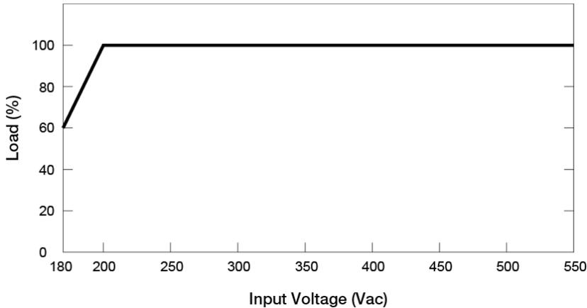
■ No output power de-rating for the input voltage range from 200Vac to 550Vac
