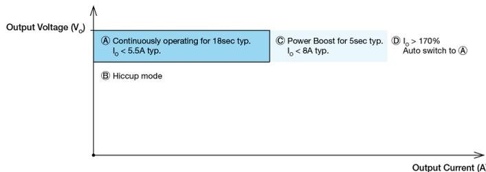
It is not recommended to prolong the duration of output current when it is <125% but >100%, since it may cause damage to the PSU.
