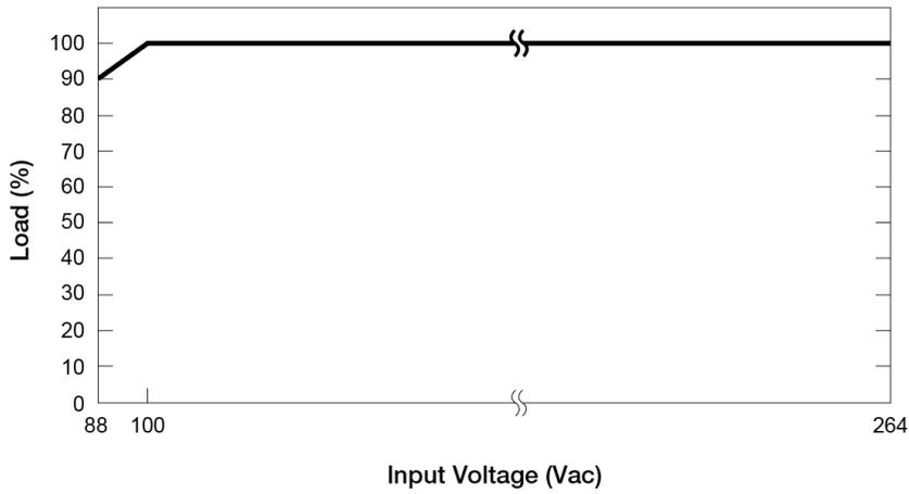
■ Output power de-rating for the AC input voltage range, refer to Fig. 6.
