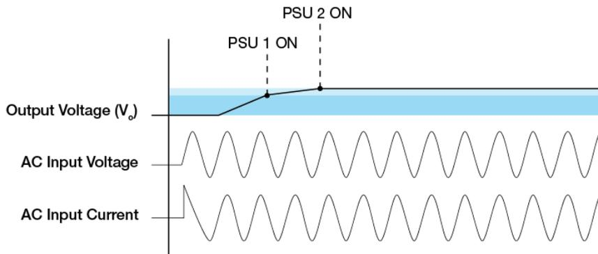
The turn ON would be non-monotonic as the power supply with the fastest startup time and rise time will turn on first. As a result, the combined output voltage waveform of the 2 power supplies connected in series will include a step.
