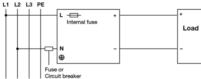
Fig. 15 2 of 3 Phase System Input Operation Connection Diagram
