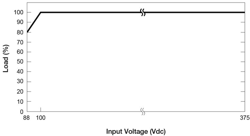
■ Output power de-rating for the DC input voltage range, refer to Fig. 7.
