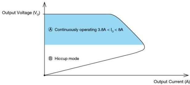
The Overload Protection (OLP) is limited at output power of less than 100W according to safety requirements.
