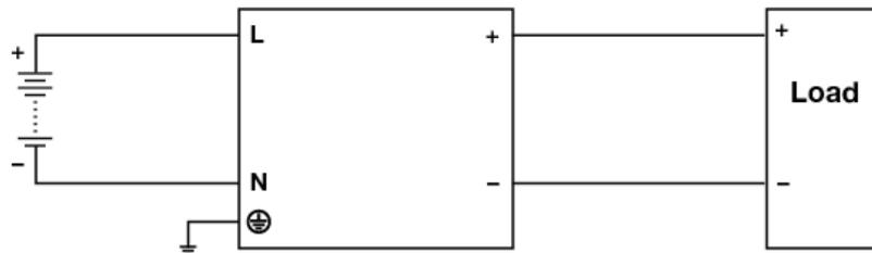
Fig. 6 DC Input Operation Connection Diagram
