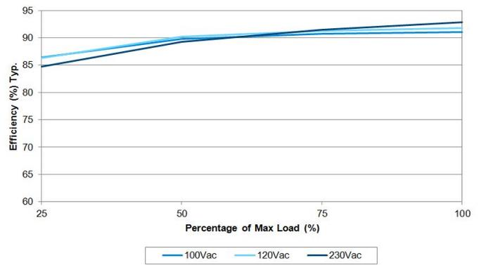
Fig. 2 Efficiency Vs Output Load at 24V
