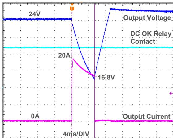
Fig. 8.3 APB 400% of nominal output current for 5ms
