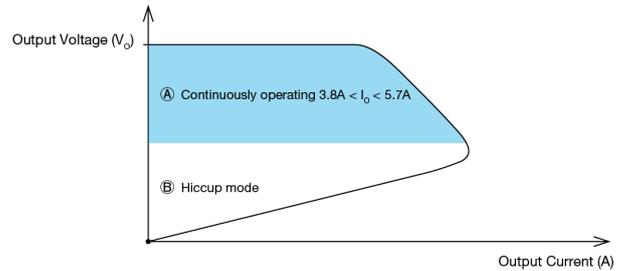
Additionally, if the  $I_o$  is  $> 102\sim 108\%$  for a prolonged period of time (depending on the load), the Over Temperature Protection (OTP) will be activated due to high temperature on critical components. The power supply will then go into "Latch mode" until the PSU cools down and the AC power is recycled.
