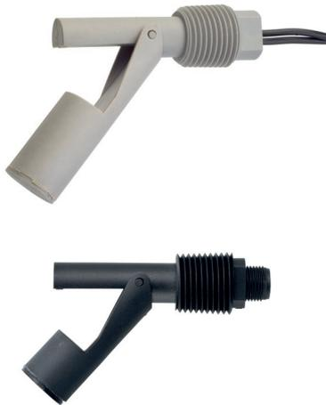
The RSF80 series are designed for mounting through the wall of a tank, via 1/2"NPT thread without requiring access to the inside of the tank.
