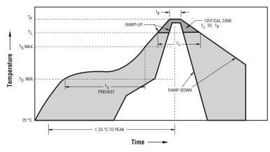
$\begin{aligned} & \text{Ramp-up rate} = 3 \text{ °C/sec. max.} \\ & \text{Ramp-down rate} = 6 \text{ °C/sec. max.} \\ & \text{T}_L = 217 \text{ °C} \qquad t_L = 60\text{-}150 \text{ sec.} \end{aligned}$
