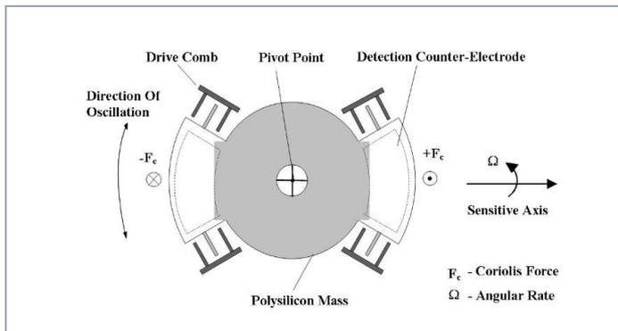
**Fig. 1: Basic layout of the sensing element of SMG061**
