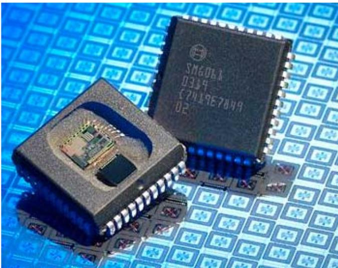
Angular Rate Sensor for Rollover Applications
