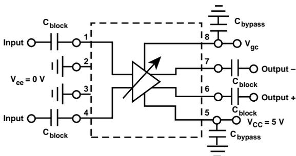
$C_{bypass} = 1000\text{ pF}$  typical
