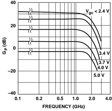
**Figure 1. Typical Variable Gain vs. Frequency.**
