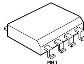
The IVA series of variable gain amplifiers is fabricated using HP's 10 GHz  $f_T$ , 25 GHz  $f_{MAX}$  ISOSAT™-I silicon bipolar process. This process uses nitride self-alignment, submicrometer lithography, trench isolation, ion implantation, gold metallization and polyimide inter-metal dielectric and scratch protection to achieve excellent performance, uniformity and reliability.
