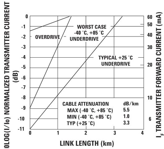
Figure 4. HFBR-14x2Z/HFBR-24x2Z Link Design Limits with 100/140  $\mu\text{m}$  Cable.
