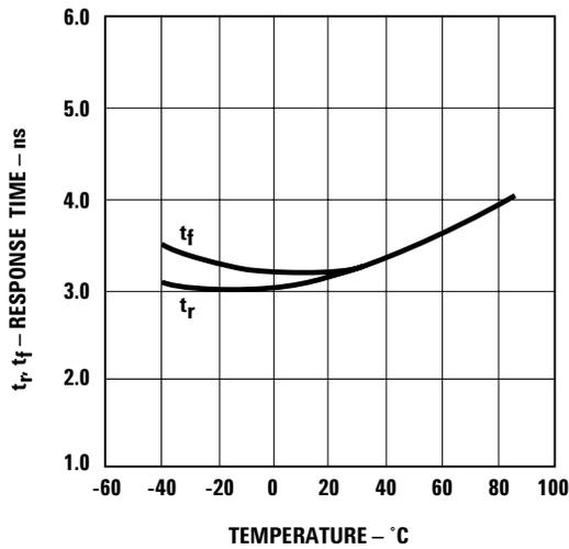
Figure 17. Typical Rise and Fall Times vs. Temperature.
