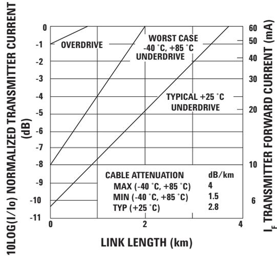
Figure 3. HFBR-1414Z/HFBR-2412Z Link Design Limits with 62.5/125  $\mu\text{m}$  Cable.
