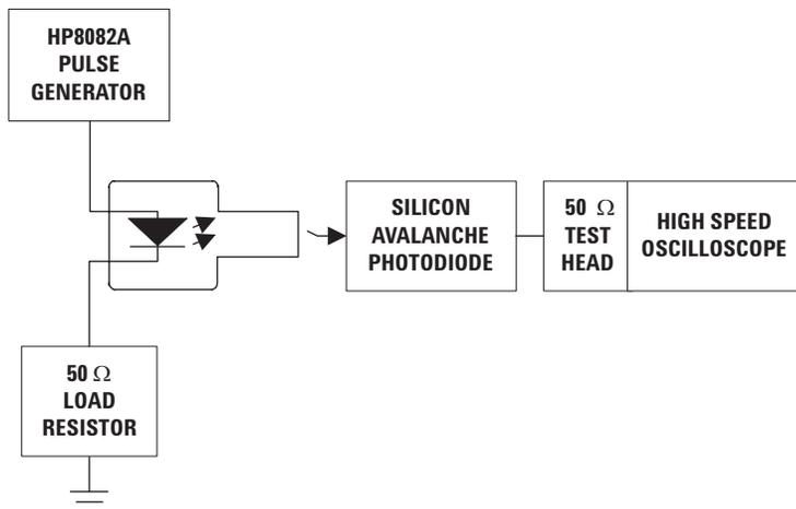
Figure 12. Test Circuit for Measuring  $t_r$ ,  $t_f$ .
