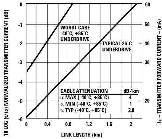
Figure 5. HFBR-14x4Z/HFBR-24x2Z Link Design Limits with 50/125  $\mu\text{m}$  Cable.
