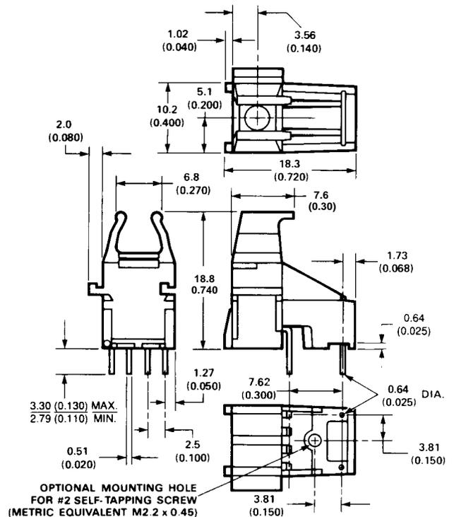
Versatile Link Printed Board Layout Dimensions
