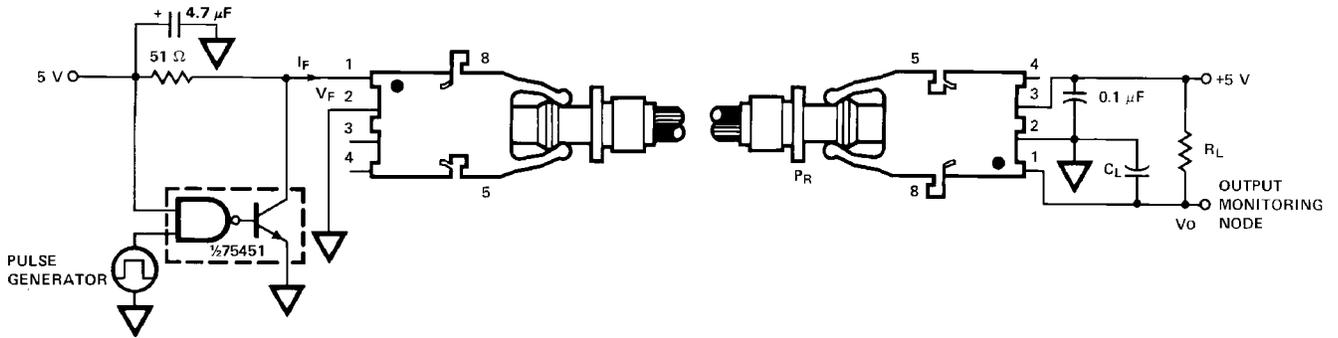
Figure 5. 5 MBd propagation delay test circuit.
