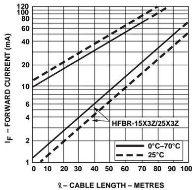
Figure 21. Guaranteed system performance with standard cable.
