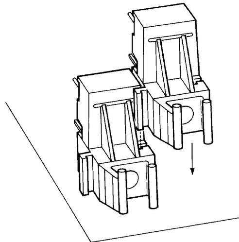
Figure 1. Interlocked (stacked) horizontal or vertical packages.
