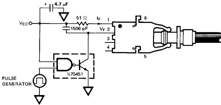
Figure 16. 1 Mb/s propagation delay test circuit.
