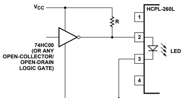
Figure 16. TTL open-collector/open drain gate drive circuit.
