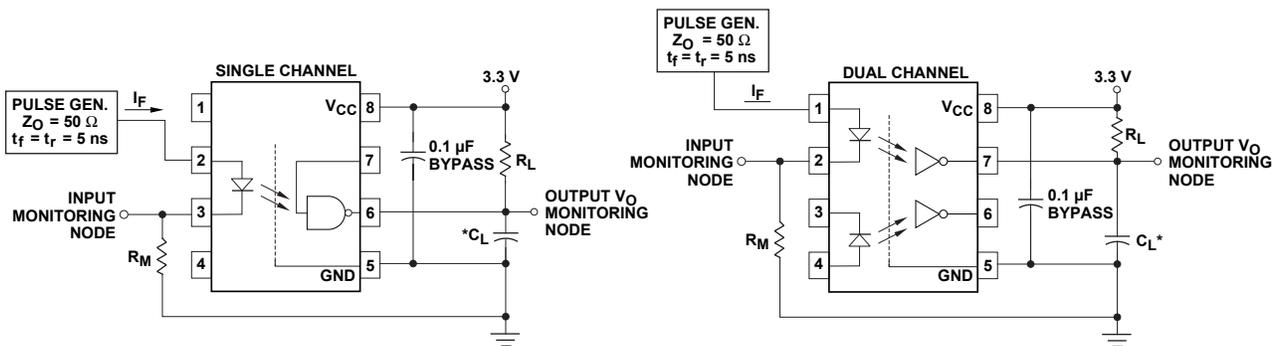
\*C<sub>L</sub> IS APPROXIMATELY 15 pF WHICH INCLUDES PROBE AND STRAY WIRING CAPACITANCE.
