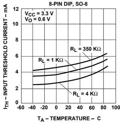
Figure 2. Typical input threshold current vs. temperature.
