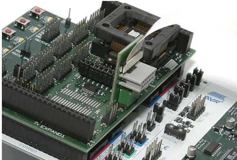
Figure 4-3: JTAG programming the AVR
