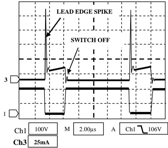
Figure 5. Lead Edge Spike Ch1: V<sub>DRAIN</sub>, Ch3: I<sub>DRAIN</sub>
