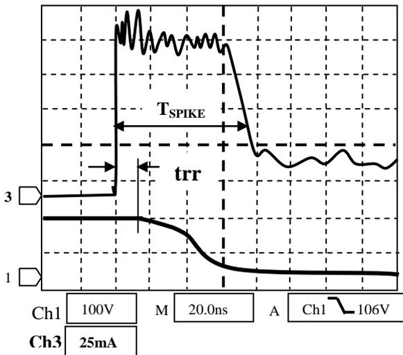
Figure 6. Switch-Off Transition. Ch1: V<sub>DRAIN</sub>, Ch3: I<sub>DRAIN</sub>
