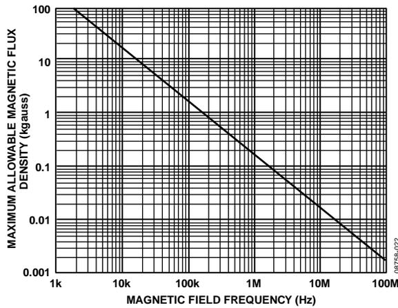
Figure 25. Maximum Allowable External Magnetic Flux Density
