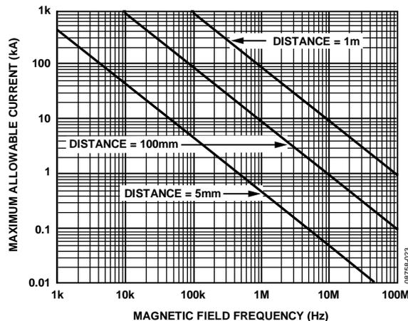
Figure 26. Maximum Allowable Current for Various Current-to-ADuM5401W/ADuM5402W/ADuM5403W Spacings
