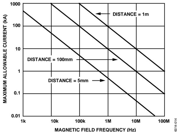
Figure 14. Maximum Allowable Current for Various Current-to-ADuM524x Spacings
