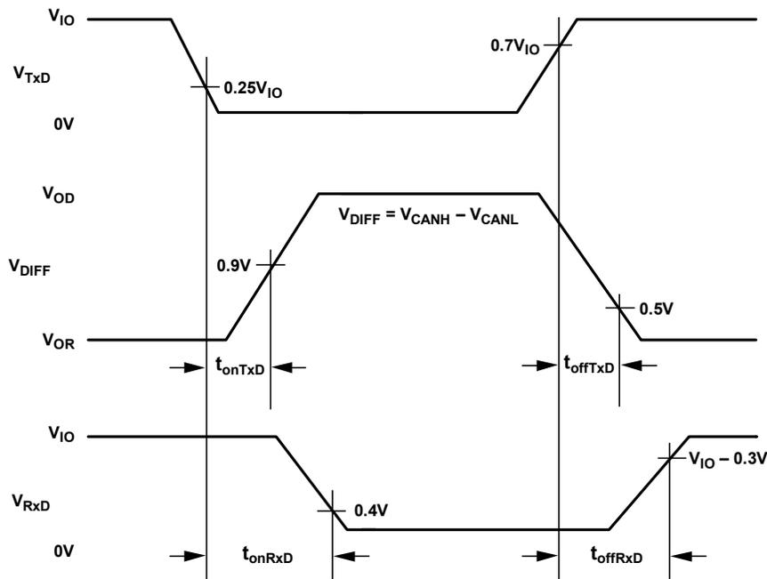
Figure 2. Driver Propagation Delay, Rise/Fall Timing
