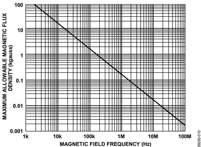
Figure 26. Maximum Allowable External Magnetic Flux Density
