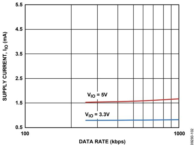
Figure 7. Supply Current,  $I_{IO}$  vs. Data Rate
