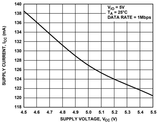
Figure 19. Supply Current,  $I_{CC}$  vs. Supply Voltage  $V_{CC}$
