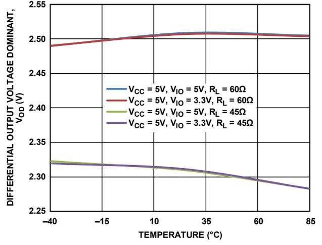
Figure 15. Differential Output Voltage Dominant vs. Temperature
