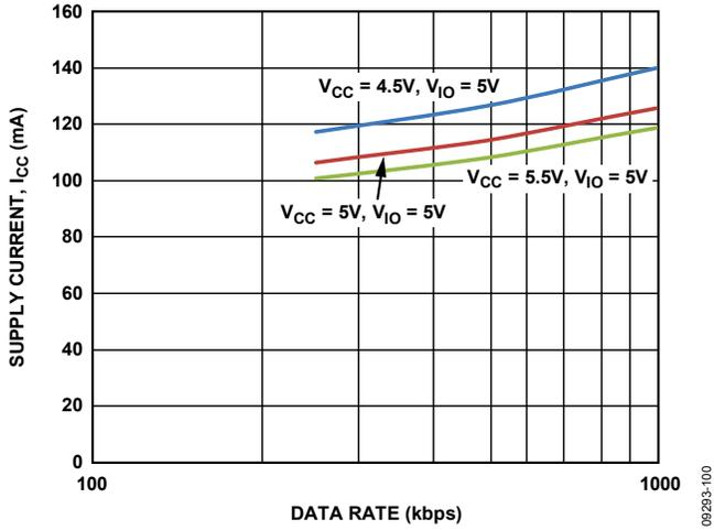
Figure 5. Supply Current,  $I_{CC}$  vs. Data Rate
