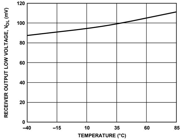
Figure 21. Receiver Output Low Voltage vs. Temperature
