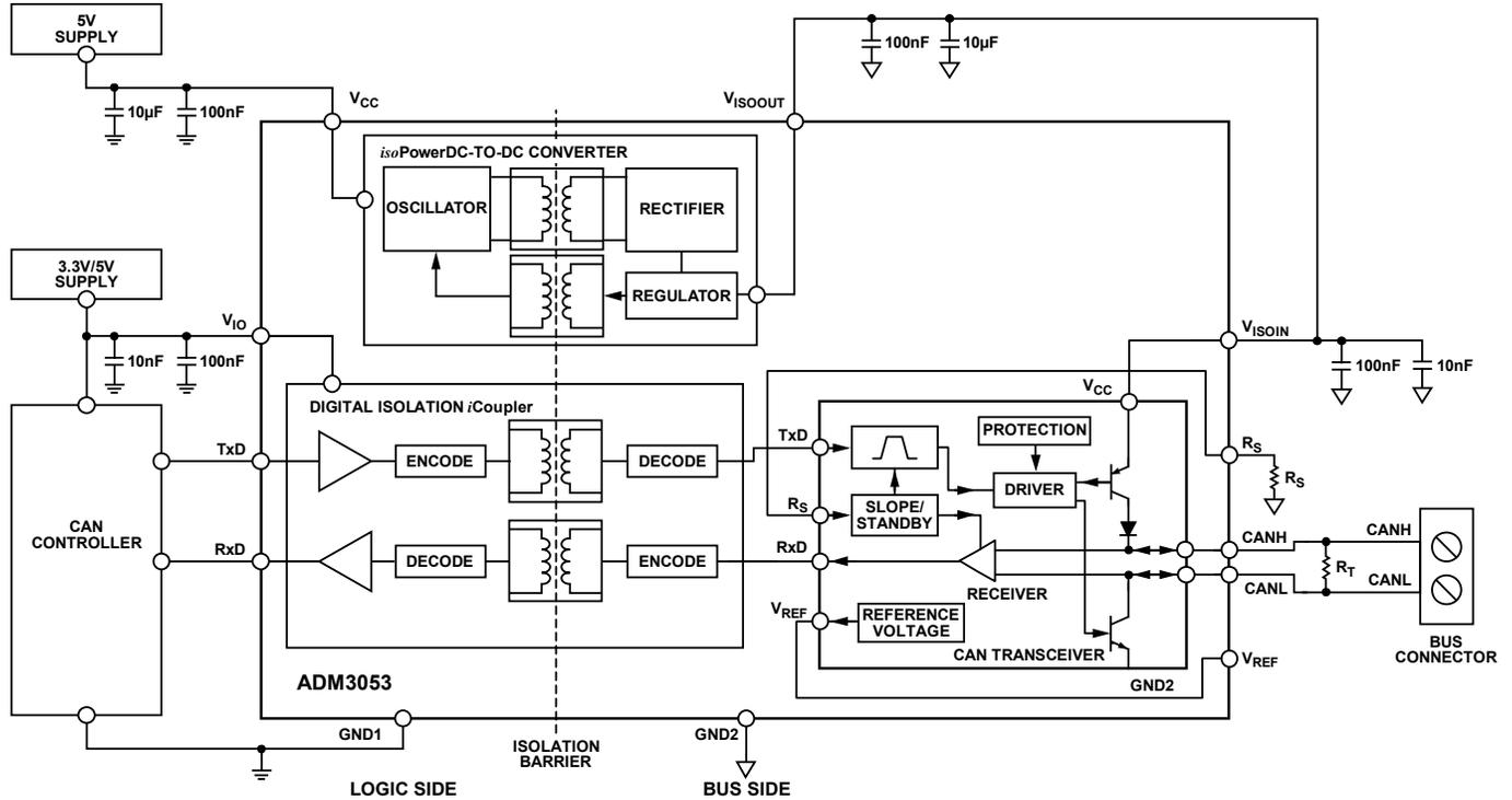
Figure 32. Example Circuit Diagram Using the ADM3053
