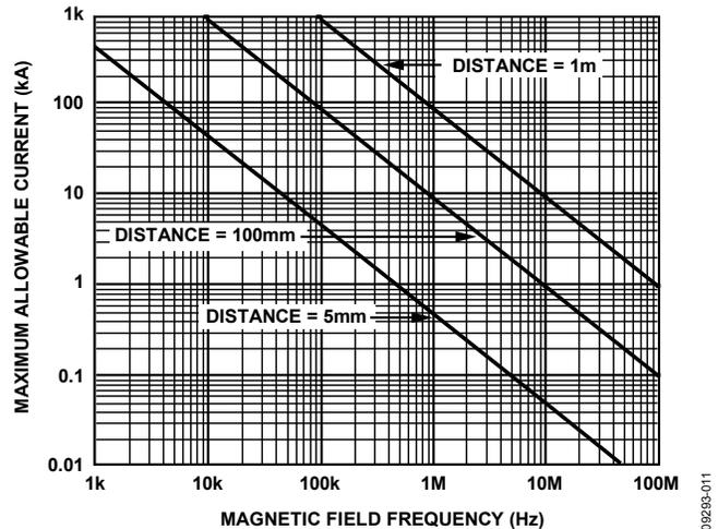
Figure 27. Maximum Allowable Current for Various Current-to-ADM3053 Spacings
