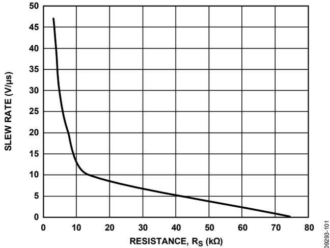
Figure 6. Driver Slew Rate vs. Resistance,  $R_S$
