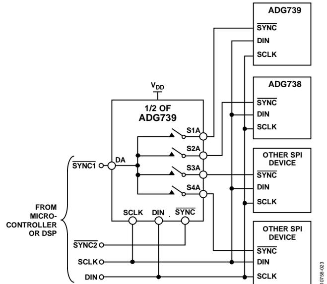
Figure 30. Addressing Multiple Serial Devices Using an [ADG739](#)
