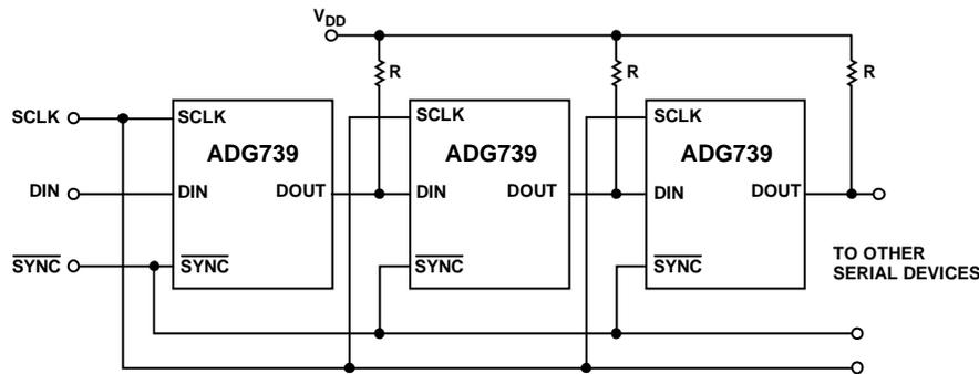
Figure 31. Multiple [ADG739](#) Devices in a Daisy-Chained Configuration
